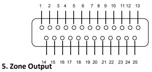
The 1-10 hot ends for CH1-CH10 11-20 for Common ends
