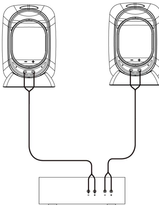
Connect the speaker terminals to the matching terminals of your amplifier: the "+" of the speaker (red) with the "+" of the amplifier, and the "-" of the speaker (black) with the "-" of the amplifier.
